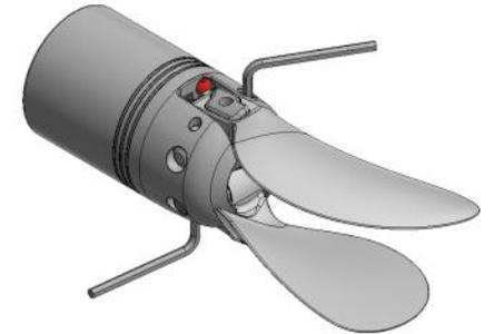
**7** Release both anchor bolts approx. 1/8 turns counter clockwise (45 degrees). Check the function, i.e. work blades open and folded to insure ease of operation.
