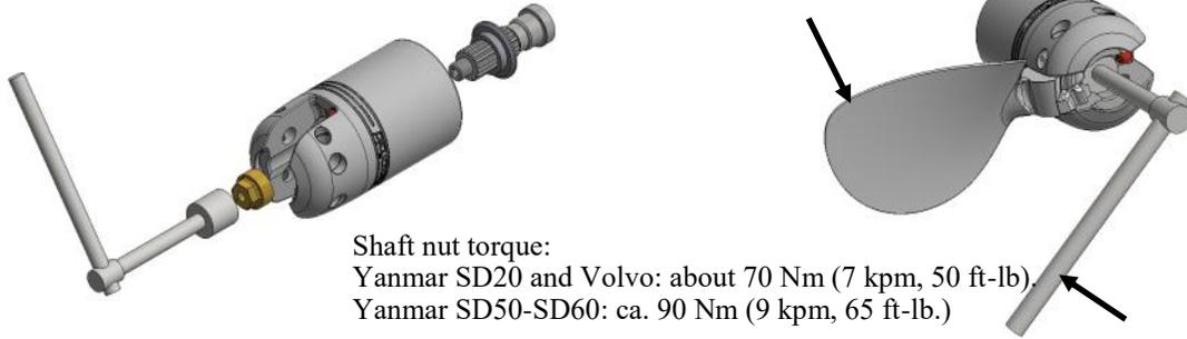
**2** Slide tab washer (5) on to shaft nut locking screw (6); screw in through hole in the shaft nut into end of shaft and tighten firmly; If using torque wrench tighten to about 15 Nm; (1,5 kpm, 10.8 ft-lb.)
