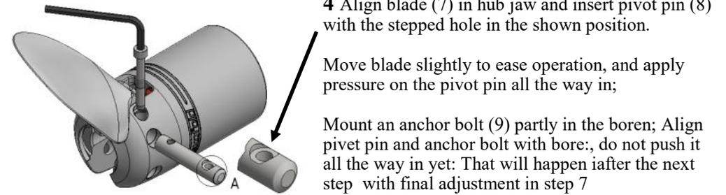
**5** Insert next blade (7), pivot pin (8) and anchor bolt (9). Engage thread as soon as both blades, pivot pins and anchor bolts are in place. Tighten light and check function. Final tightening will be done in step 6 with final adjustment in step 7:
