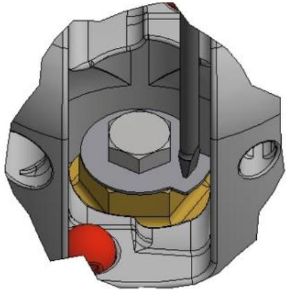
**3** Again using a straight screw driver or similar: Bend side of tab washer up over hex on the shaft nut locking screw (6). This along with the pre-applied thread locker on shaft nut locking screw will prevent it from backing out.
